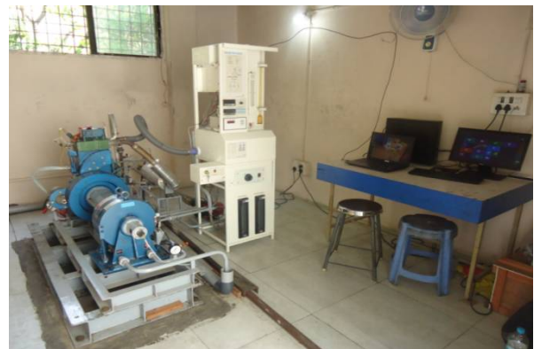
Fig.2.Computerised Engine setup for Experiment
